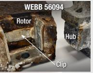
The patented Webb design features a stainless steel clip that adds a protective barrier between the rotor and hub.
